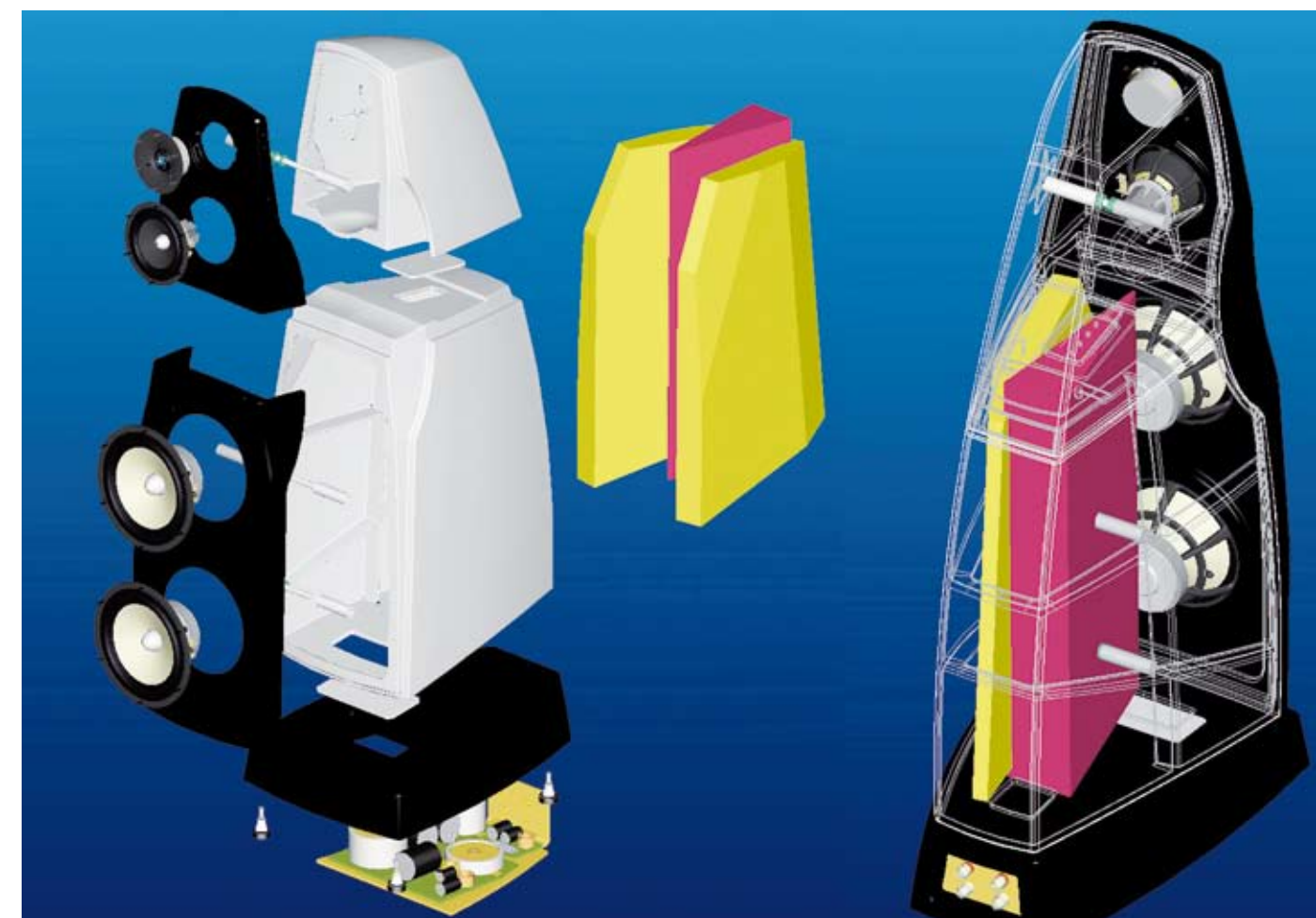
The different sized parts of the housing are additionally stabilised by horizontally running struts. Wedges made of rock wool (red and yellow) fill the cavities. The frequency separating filter sits on its own in the base.
